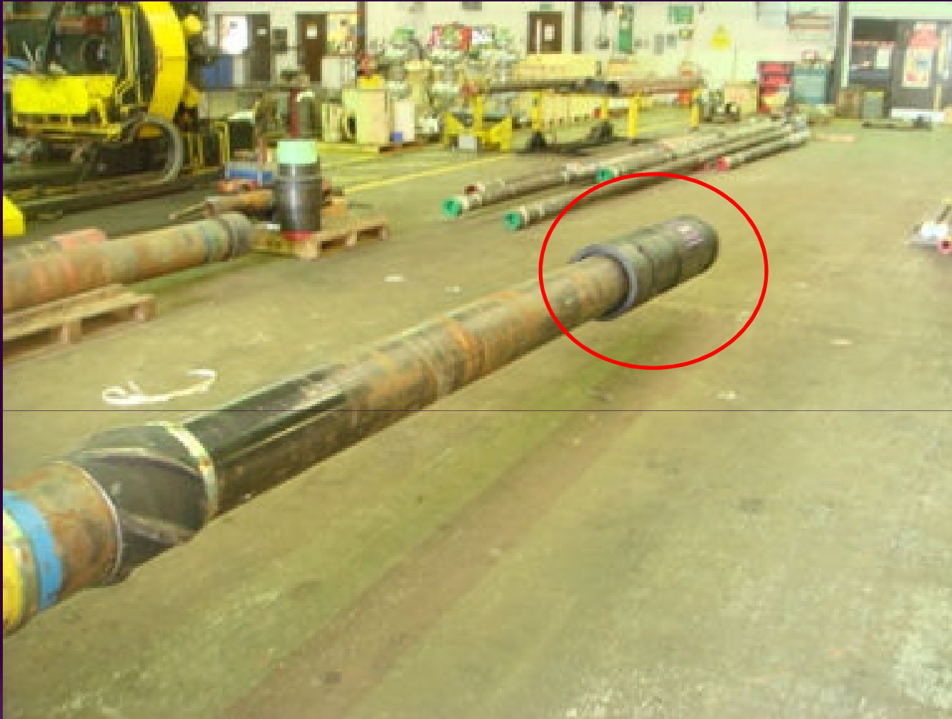
9.5/8" FloatCHECKER PT installed over a float shoe on end of joint
